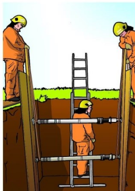
Safe zone in a trench
