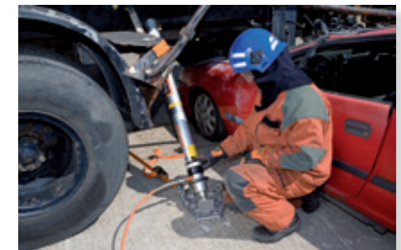
Heavy vehicle stabilization with hydraulic Locknut strut.
