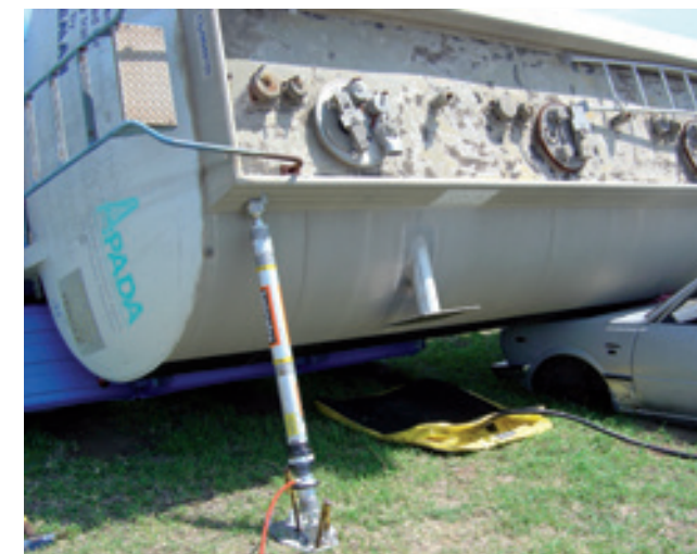
Pneumatic Auto-lock strut used for follow-up shoring in heavy vehicle lifting operations.
