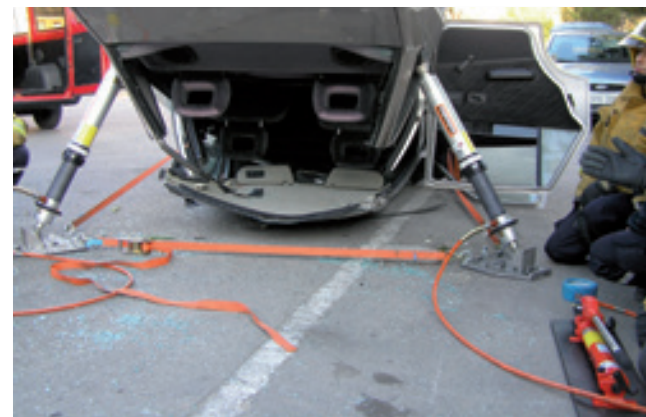
Light vehicle stabilization with hydraulic Locknut struts.
