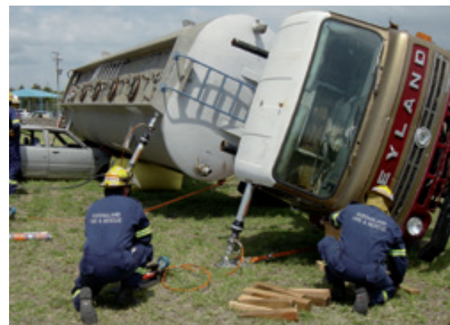
Hydraulic Auto-lock strut used for heavy vehicle lifting and shoring.
