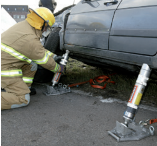
Vehicle stabilization with manual Locknut struts.
