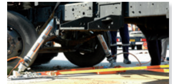
Heavy vehicle stabilization with hydraulic Locknut strut.
