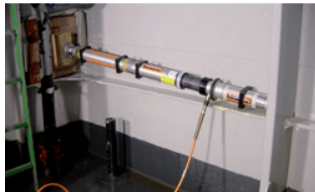
Hydraulic-powered struts used together with extensions, heads and timber to seal a leak inside a marine ship.
