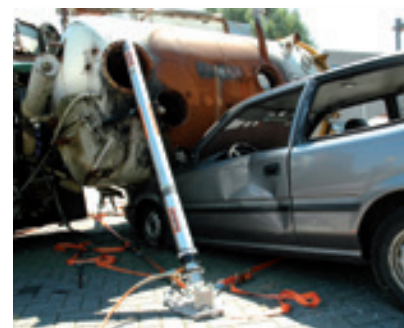
Light vehicle stabilization with hydraulic Locknut struts.
