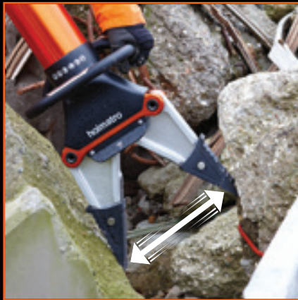
Built-in Speed Valve When unloaded, the arms open quickly to the desired distance to speed up spreader positioning.
